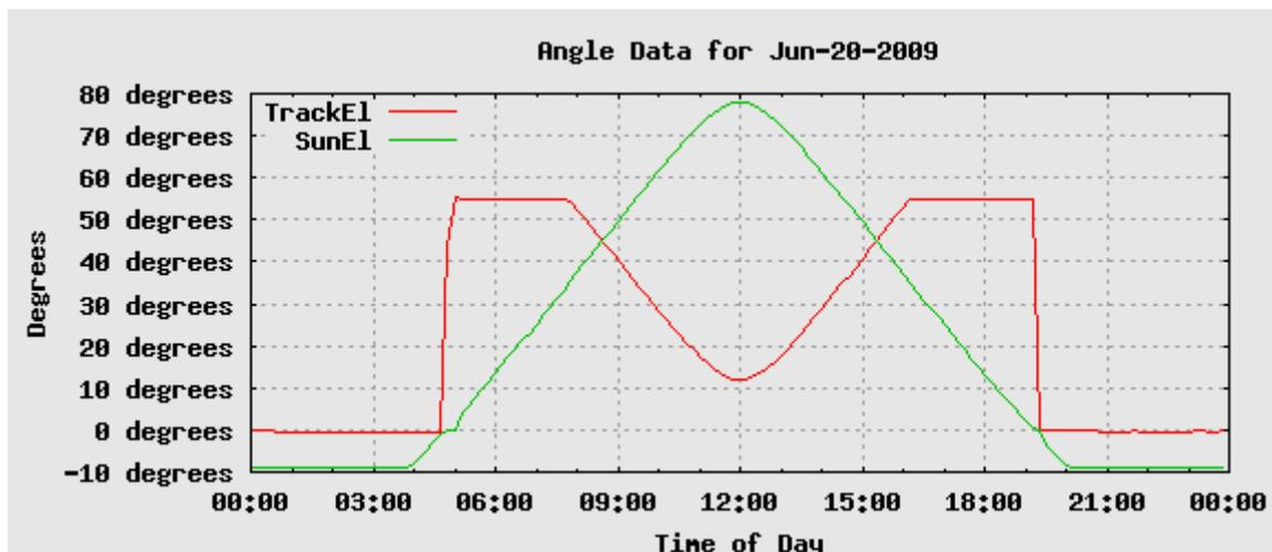
Figure 2, Graphical view Daily Solar Tracker Elevation
