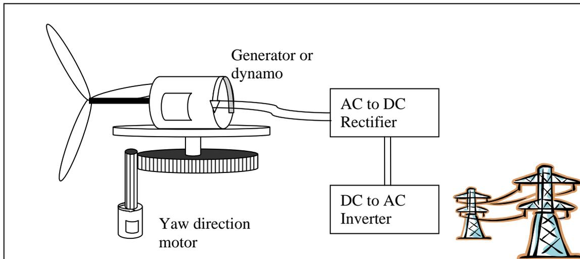
Figure 1: simplified wind turbine
