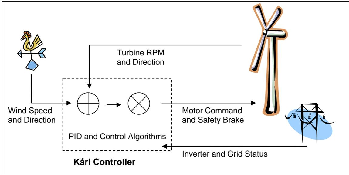
Figure 3: wind turbine control block diagram
